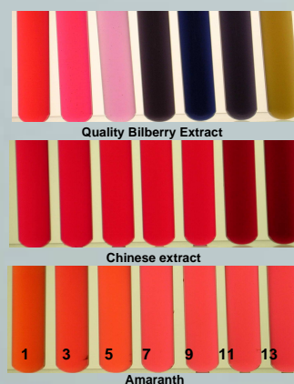
Figure 6: pH colour dependence of Anthocyanins but not amaranth (numbers are pH values)
